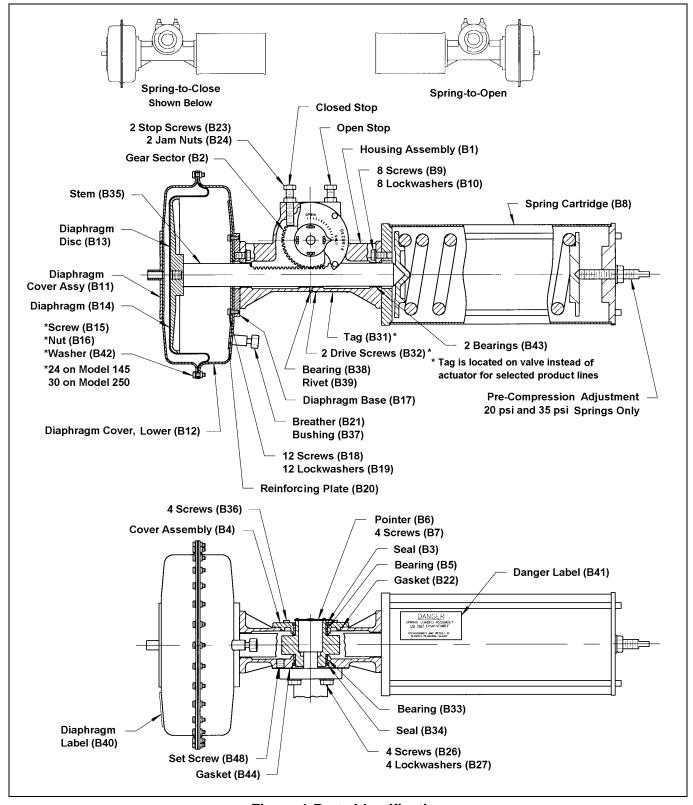
**Figure 1-Parts Identification**
