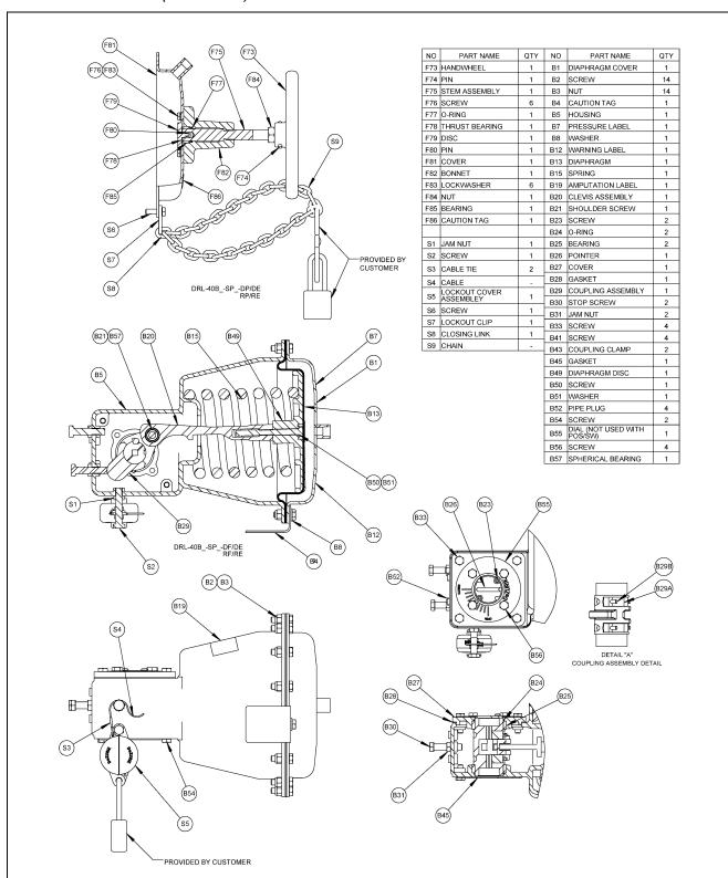
Figure 5—Lockable Model, Parts Identification
