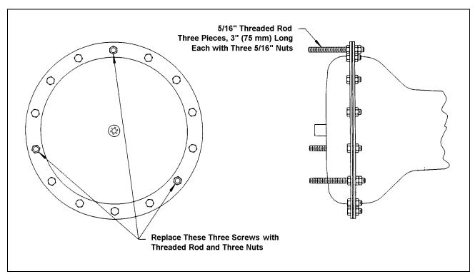
Figure 4—Stud Requirements For Diaphragm Cover Removal
