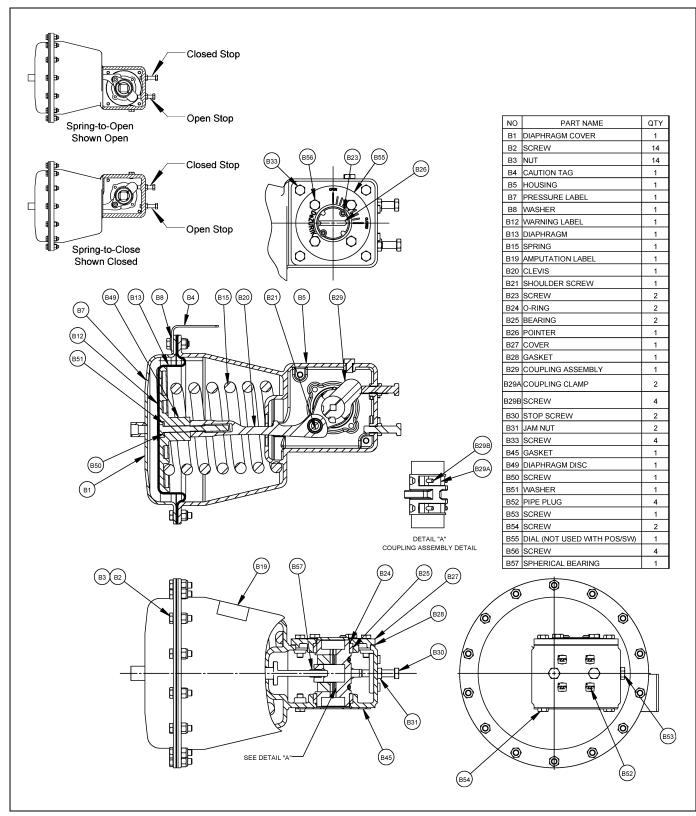
Figure 1—Parts Identification
