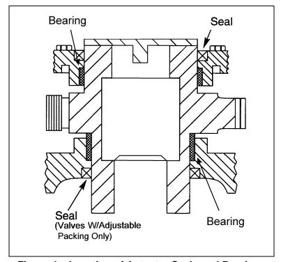
Figure 4 – Location of Actuator Seals and Bearings
