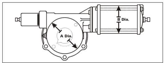
Figure 1 - Actuator Identification
