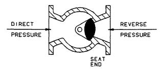
Figure 2 – Pressure Direction
