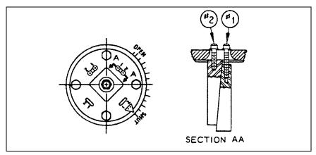
Figure 3 – 24" thru 36" Key and Lockscrew Arrangement
