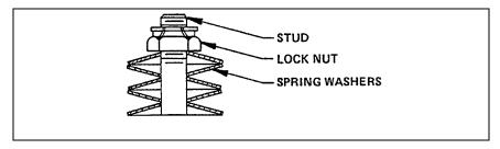
Figure 4—Spring Washer Stackup
