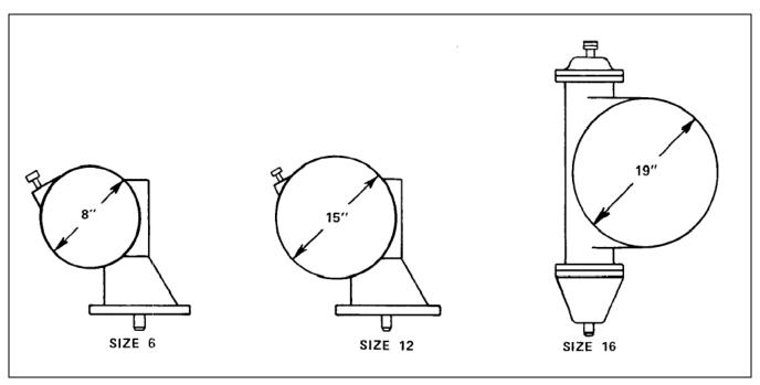
Figure 1— G-Series Actuator Identification
