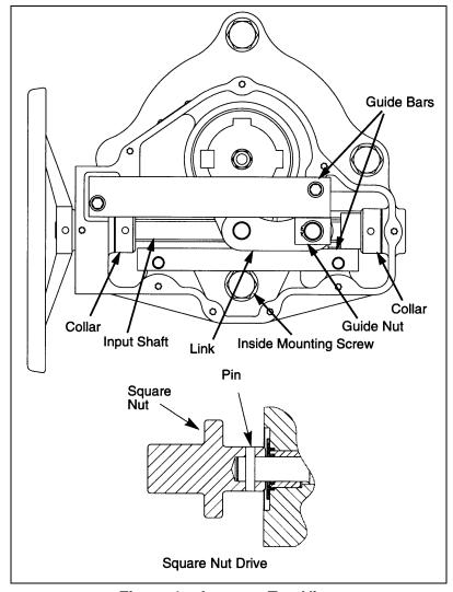
Figure 1—Actuator Top View
