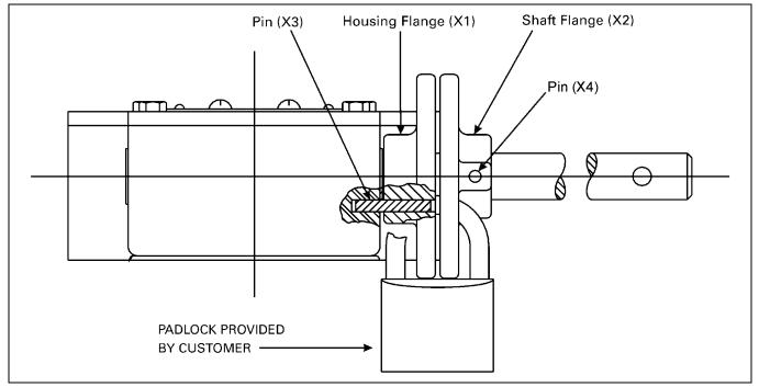
Figure 6—Lockout Parts
