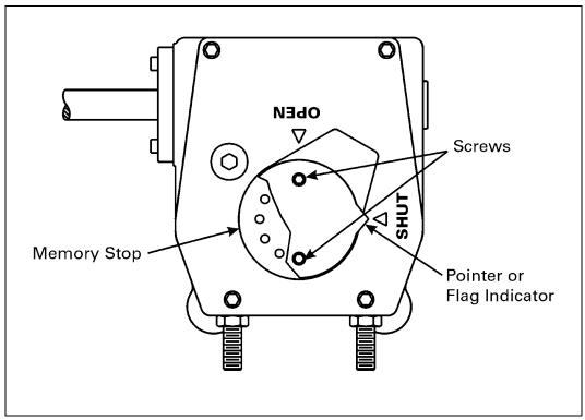
Figure 7—Memory Stop (MG-7 and MG1012)
