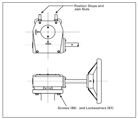
Figure 1— Component Identification
