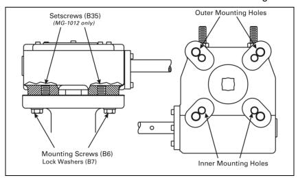
Figure 2 — Mounting Screw Locations
