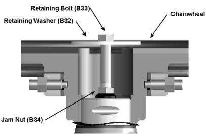
FIGURE 2—Detailed View of Chainwheel Retaining Components
