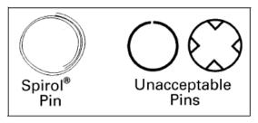
FIGURE 1– Acceptable and Unacceptable Pin Styles
