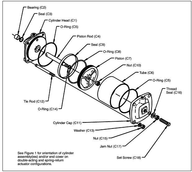
Figure 3—Double-Acting Cylinder Assembly
