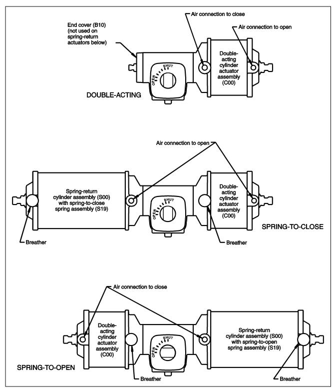
Figure 1—R1 PowerRac™ Actuator Configurations
