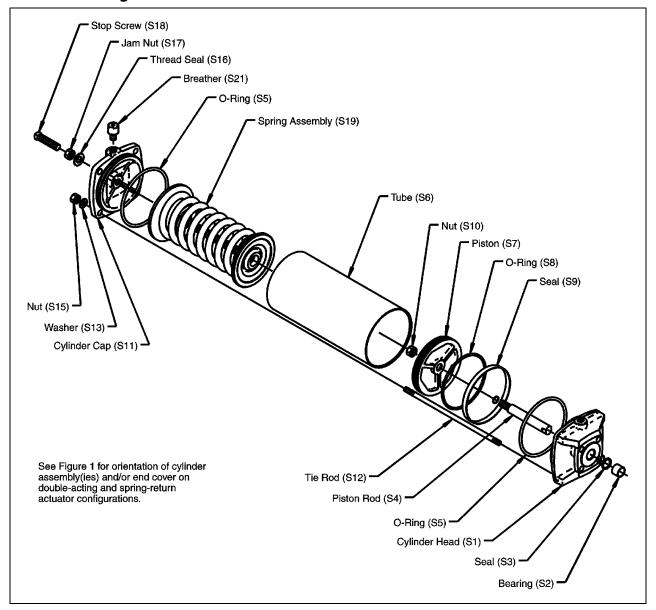
Figure 4—Spring-Return Cylinder Assembly
