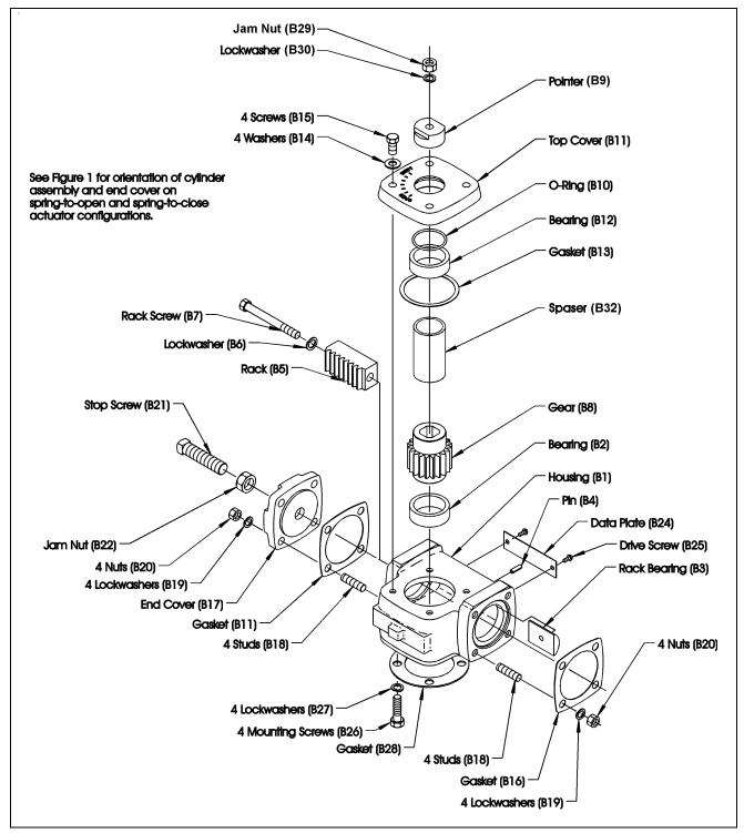
Figure 2—Actuator Assembly without Cylinder(s)
