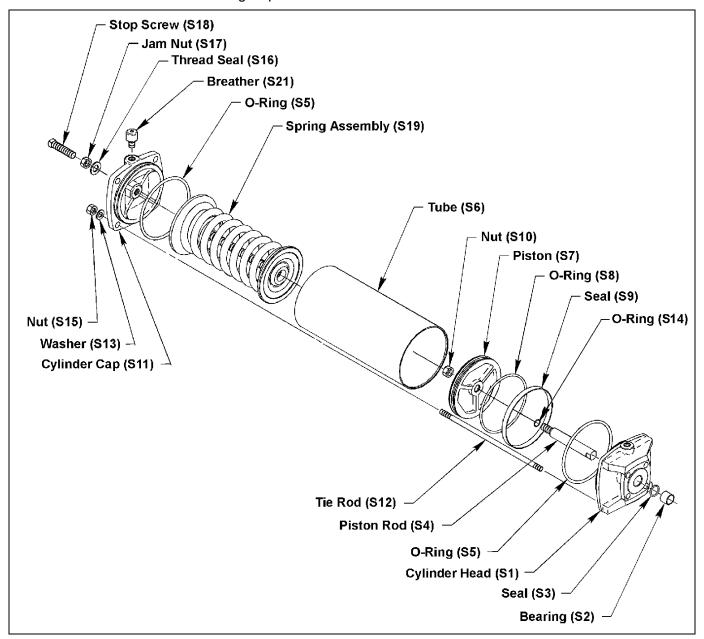
Figure 4—Cylinder Assembly
