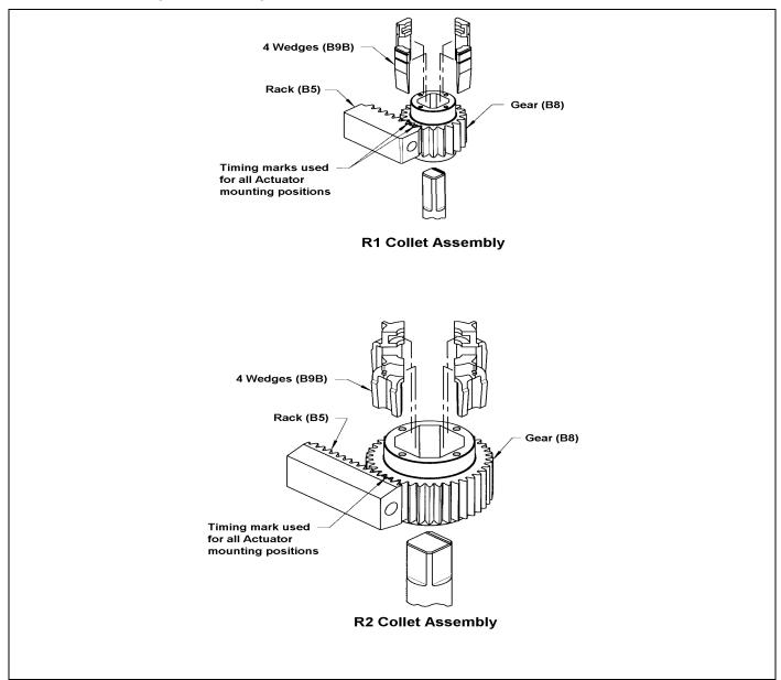
Figure 6 —Collet Assembly and Gear Alignment
