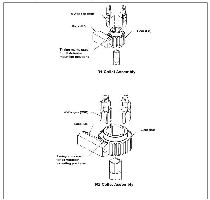
Figure 5 —Collet Assembly and Gear Alignment
