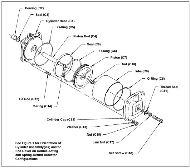
Figure 3—Double-Acting Cylinder Assembly
