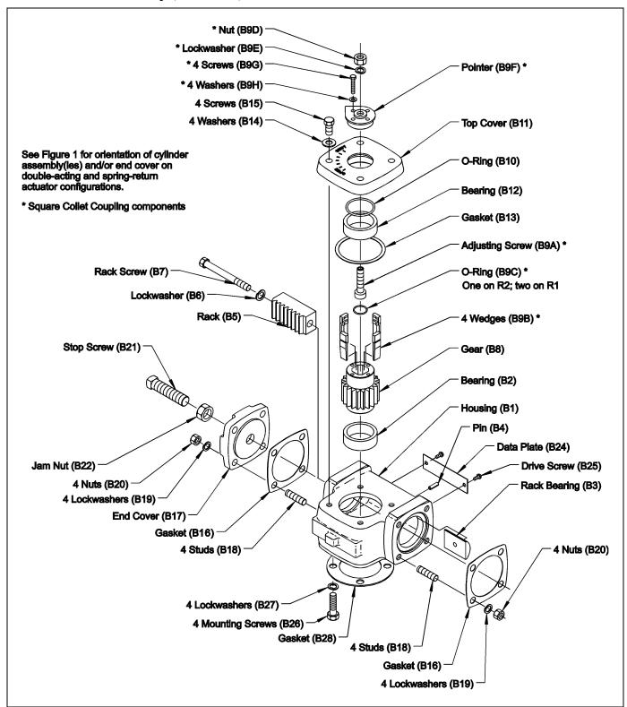
Figure 2—Actuator Assembly, Less Cylinders
