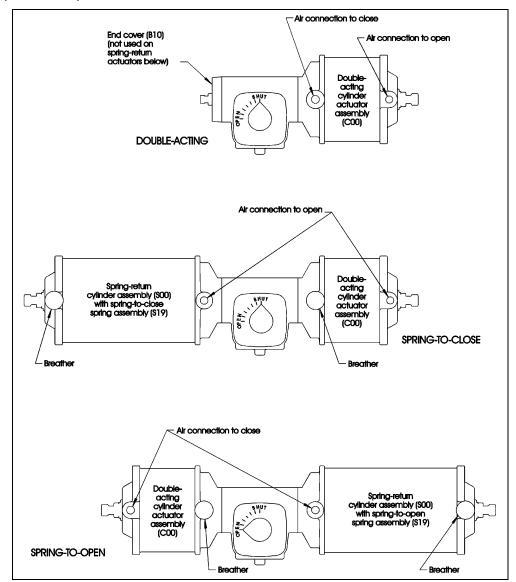
Figure 1—R1 and R2 PowerRac® Configurations
