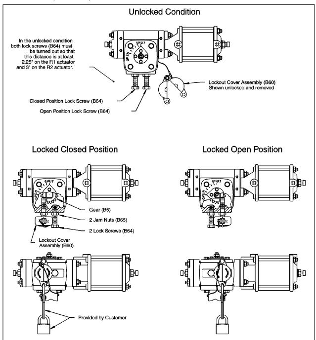
Figure 7 - Lockable Model Component Identification
