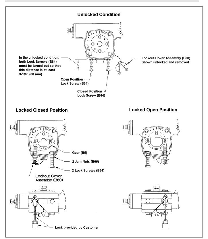
Figure 4 – Lockable Model, Component Identification
