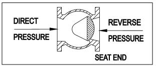
Figure 7 – Pressure Direction
