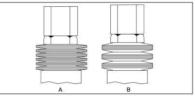
Figure 6 – Washer Stacking for Different Valve Sizes
