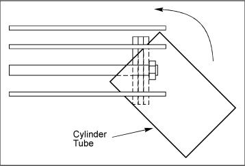
Figure 5 – Cylinder Tube Installation
