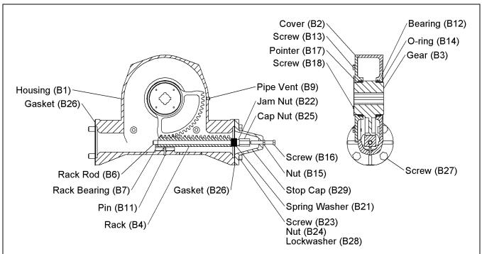
Figure 2 – Actuator Parts Identification
