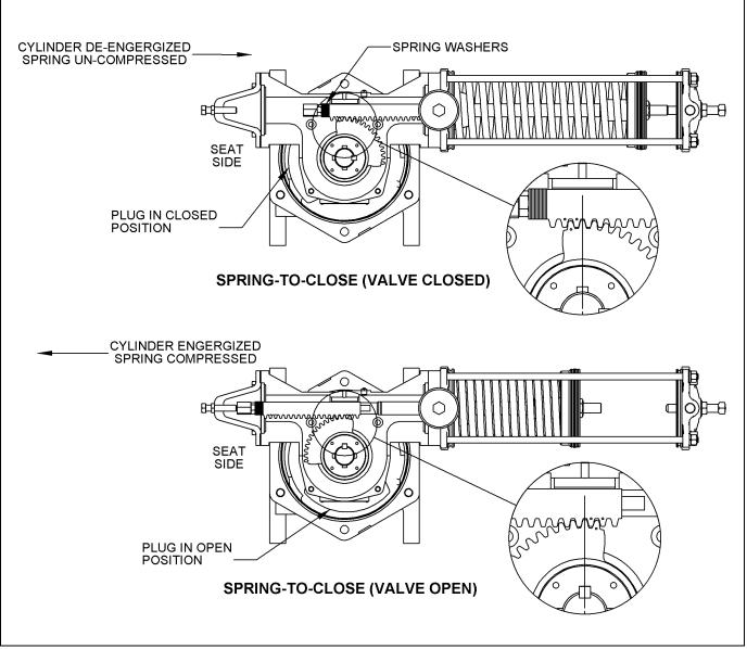
Figure 9 – Spring-To-Close Actuator (6A actuator shown)
