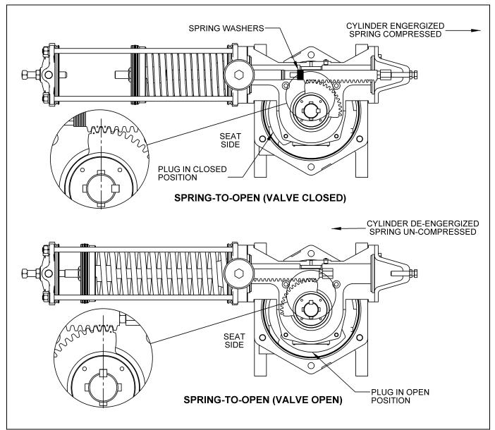
Figure 8 – Actuator Spring-To-Open (6A actuator shown )
