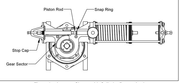
Figure 3 – Actuator Shown with Cylinder Pressurized
