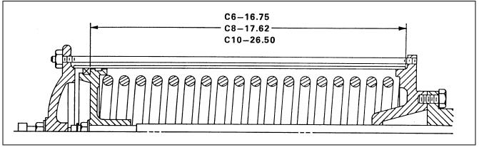
Figure 4 – Piston Length Dimension
