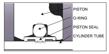
5. Remove the Cylinder Tube (C13), Piston Seal (C11) and O-ring (C12). Clean the parts and the grooves in the Piston (C10). See Figure 4.
