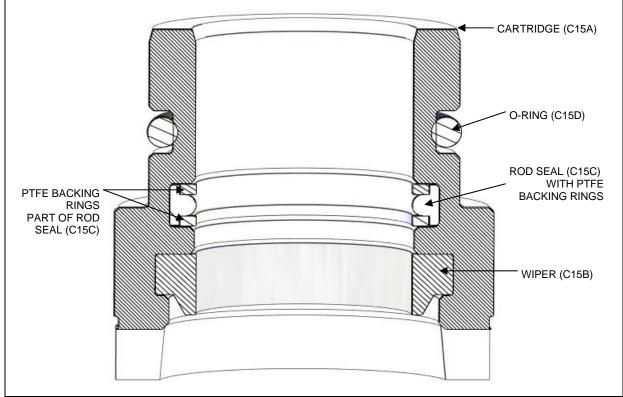
Figure 3: Cartridge Assembly (C15)
