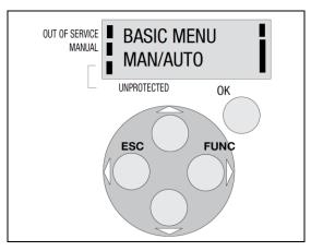
The positioner can be stroked manually using the pushbuttons. See section "Man/Auto", page 21.
