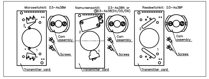
When installing the transmitter/switch card, make sure it is placed correctly over the connector pins before gently pushing it down until it rests on the supports. Secure the PC board with the two screws. Make sure the holes are centered before tightening the screws.
