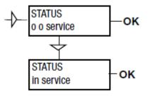
Note: When changing between In service and Out of service, the OK button must be pressed for 3 seconds.
