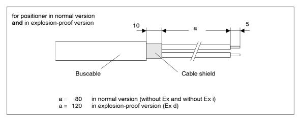
Figure 3-13 Preparation of bus cable
