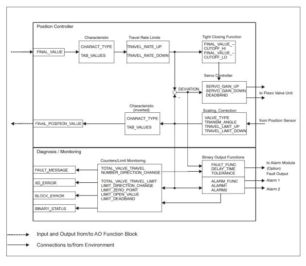
Figure 5-3 Function schematic of Analog Output transducer block
