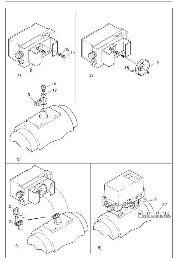
Figure 3-8 Assembly procedure (rotary actuator)
