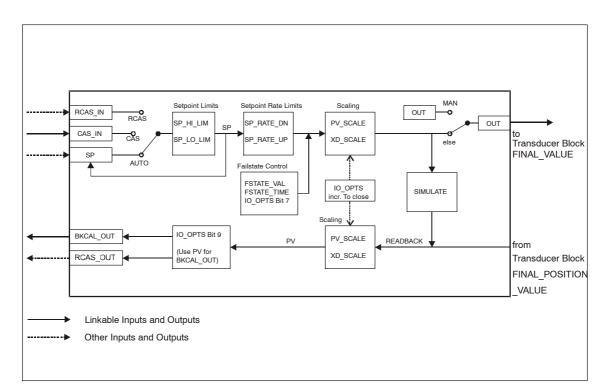
Figure 5-2 Function schematic of AO function block
