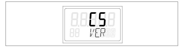
Figure 4-3 Firmware version, example: C5
