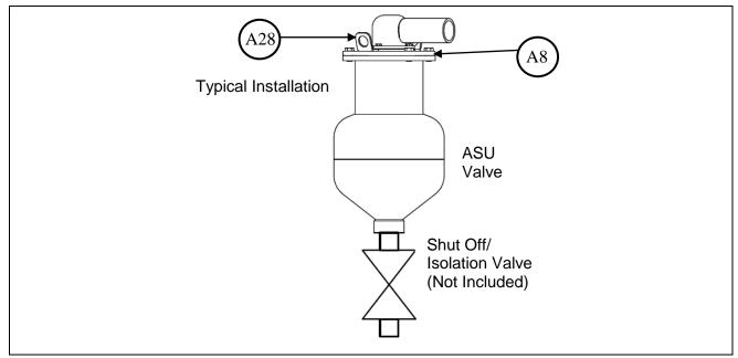
Figure 1 – Typical Installation
