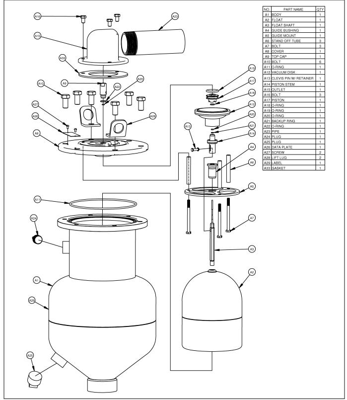
Figure 2: ASU-SCAV Part Identification (Exploded View)
