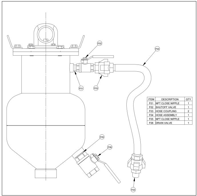
Figure 6: ASU-SCAV with Optional Backflush Attachment Parts Identification
