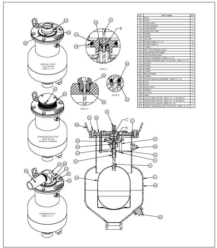
Figure 3: ASU-SCAV Part Identification
