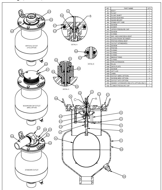
Figure 5: ASU-CAV Combination Air Valve Part Identification
