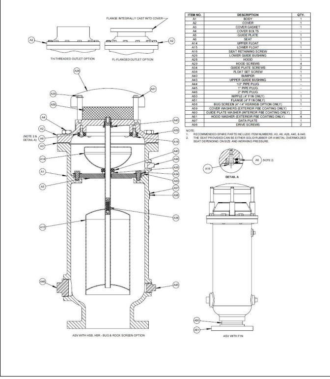
Figure 2: ASV-401 4-14" (100-355mm) Sewage Air/Vacuum Valve
