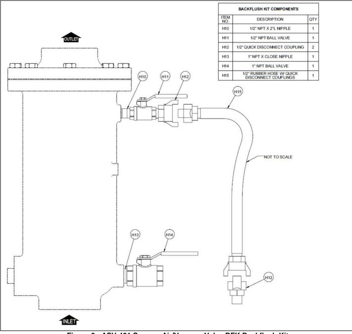
Figure 3: ASV-401 Sewage Air/Vacuum Valve BFK Backflush Kit
