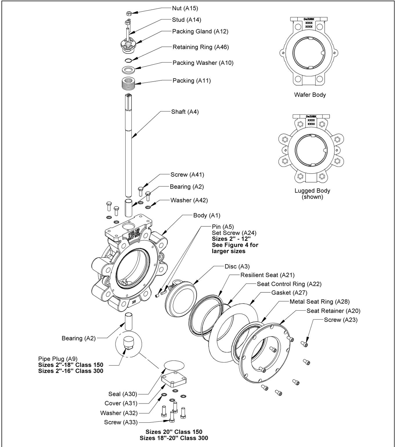
**Figure 1 – Component Identification**
