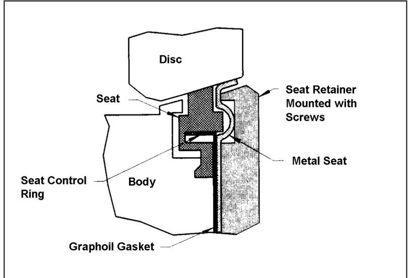
**Figure 3 — (FB) Fyre-Block Seat Options (RTS2 and TTS2)**
