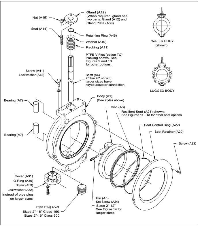
Figure 1 – Component Identification
