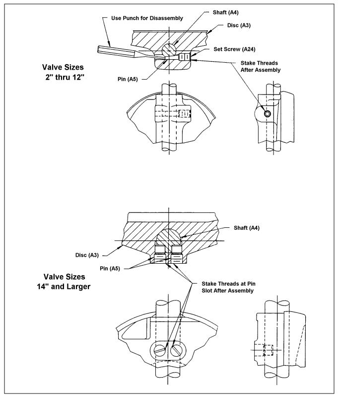
Figure 14 – Disc Pin Assembly
