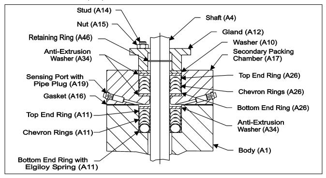
Figure 4 – Packing Option (TMD)
