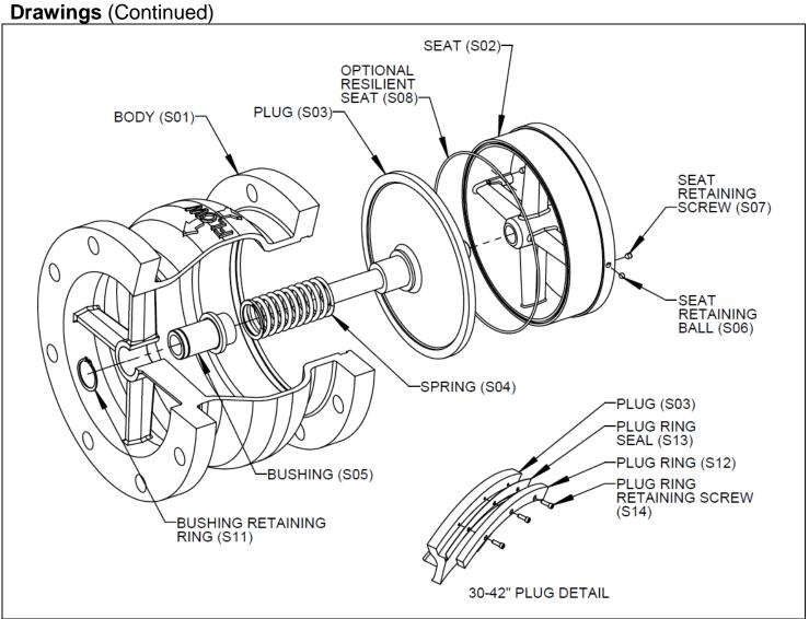
Figure 5: CSC-600A Globe Style Silent Check Valve (Exploded View)
