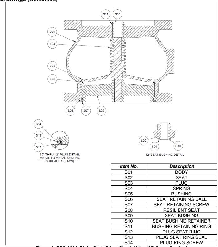
Figure 4: CSC-600A Globe Style Silent Check Valve (2D Cross Section)
