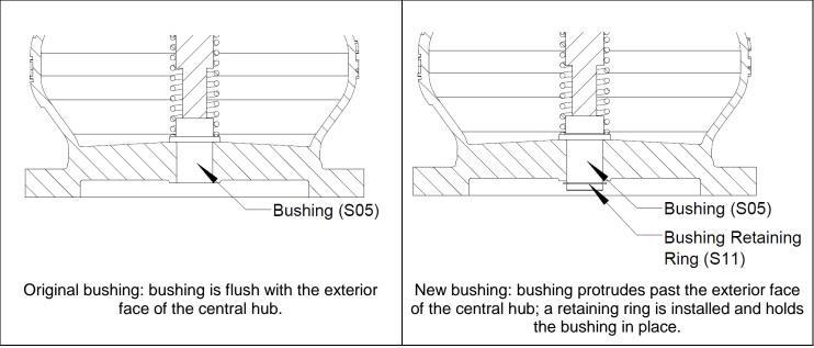
The CSC-600A Globe Style Silent Check Valve will come equipped with one of two bushings: a standalone bushing or a bushing with a bushing retaining ring.
