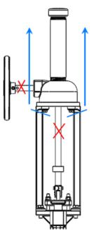
Figure 4- Knife Gate Valve with Bevel Gear Actuator, Vertical Lifting
