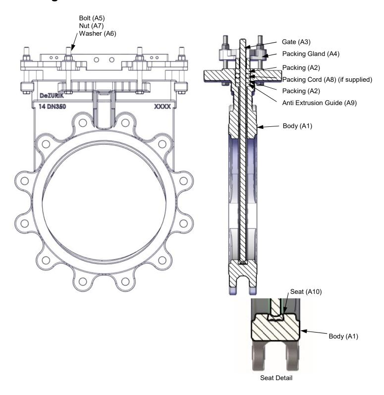
Figure 1—Component Identification
