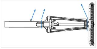
Figure 3, Knife Gate Valve with Handwheel or Chainwheel Actuator, Horizontal Lifting
