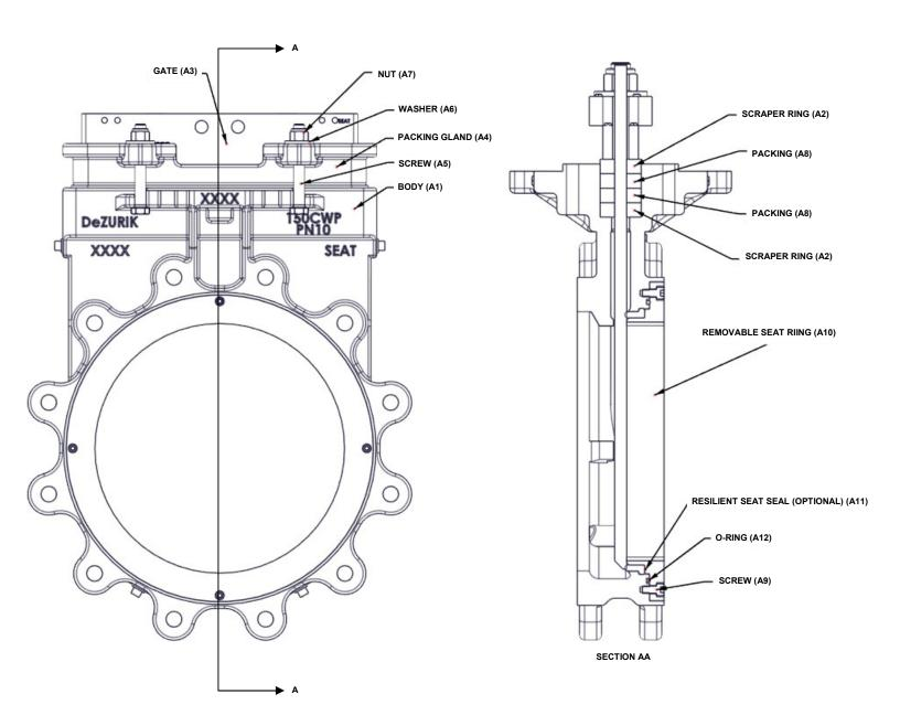
Figure 2—Component Identification
