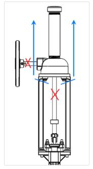
Figure 4- Knife Gate Valve with Bevel Gear Actuator, Vertical Lifting
