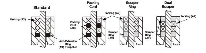
Figure 3—Packing Detail
