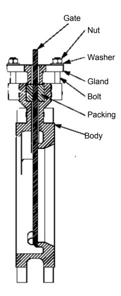
Figure 1—Component Identification
