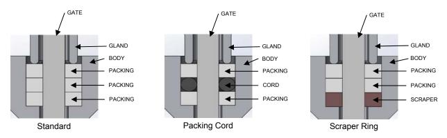
Figure 2—Packing Ring Sequence
