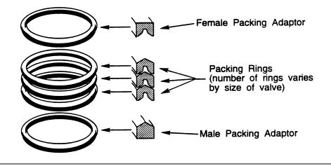
Figure 4 — Correct Packing Installation Sequence
