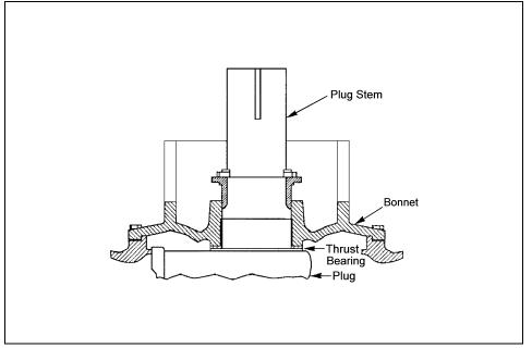
Figure 6 — Thrust Bearing Contacting Bonnet Inside of Valve
