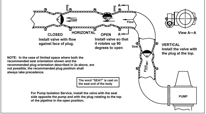
Figure 3 — Liquids with Suspended Solids
