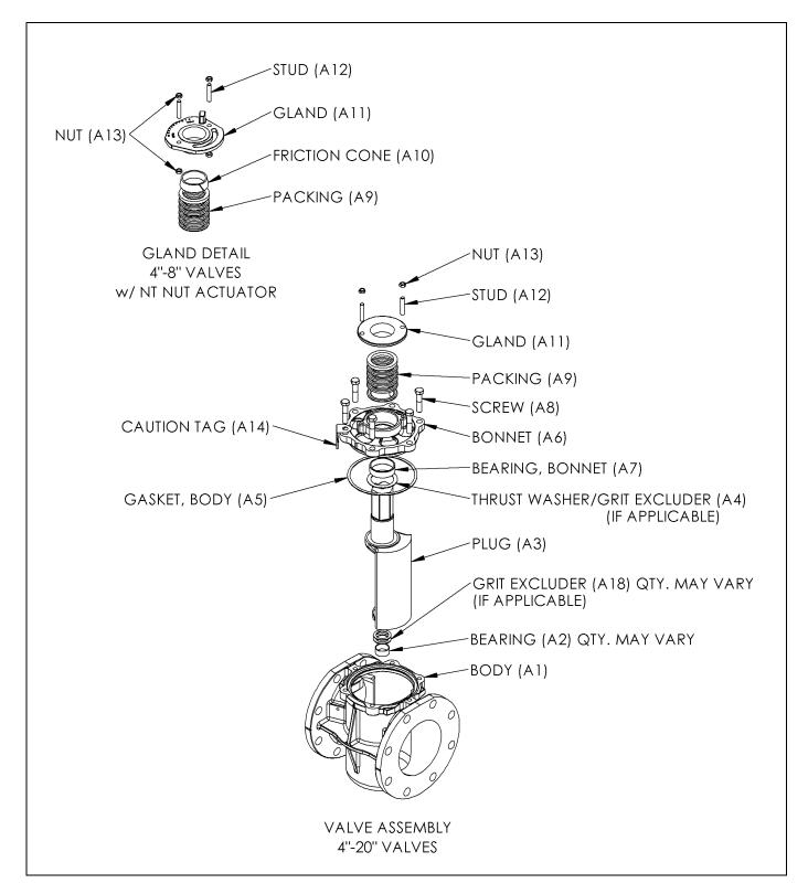
Figure 3 – Parts Identification
