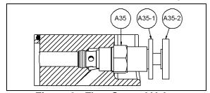
Figure 2: Flow Control Valve
