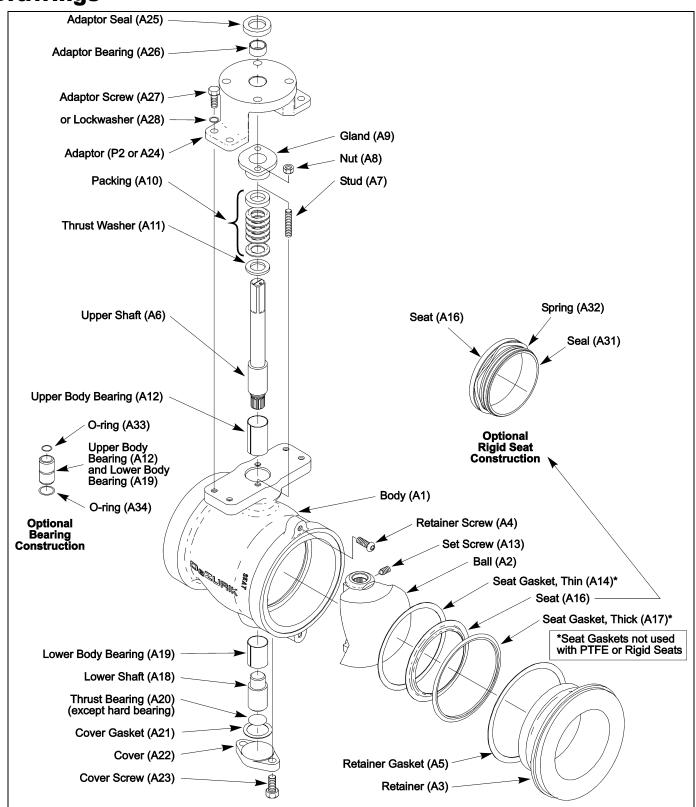
Figure 1 – Component Identification Disassembled
