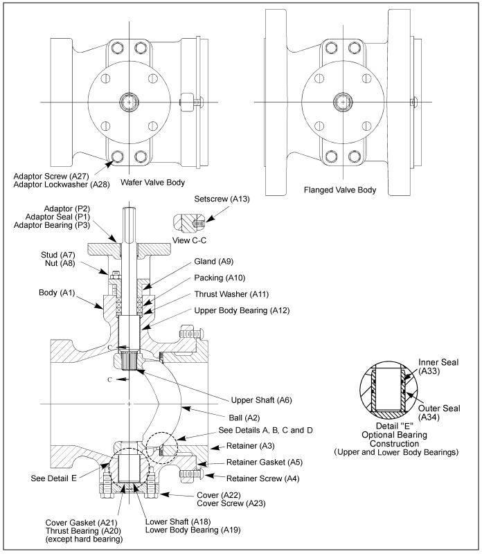
Figure 2A – Component Identification Assembled
