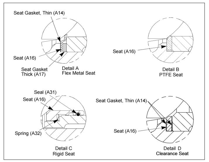
Figure 2B – Component Identification (Seat Details)
