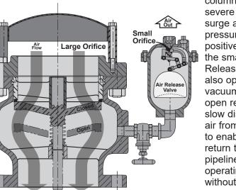
column and minimize severe pressure surge as system pressure returns to positive. Meanwhile, the small orifice Air Release Valve has also opened due to vacuum and stays open regulating a slow discharge of air from the pipeline to enable a gradual return to normal pipeline system operating pressure without damage.
