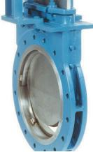
All valves are provided with 304 stainless steel guides for corrosion resistance. Gates are finish ground on both sides and edges to increase packing life. Gate guide provides rigid support for the moving gate. Gate jams at the bottom of the body hold the gate securely against the seat.
