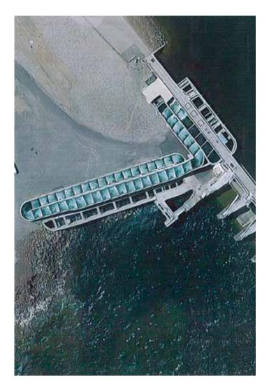
An aerial view of the fish ladder and the attraction pool. The water supply for the attraction pool is controlled with a 66" DeZURIK Eccentric Plug Valve.
