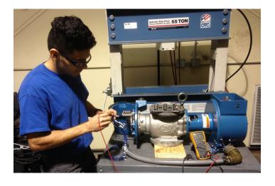
Factory-trained field service personnel perform preventative maintenance on-site during scheduled shut-downs or at a DeZURIK Service Center. Any valve performance problems are addressed. The valve motor. harmonic gear drive, control/feedback components and seals are removed, fully inspected, greased and replaced as required. The preventative
