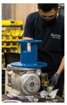
maintenance returns the valve to manufacturer's specifications. The valve is performance tested, recalibrated and verified to the satisfaction of paper mill operators.
