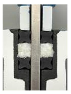
Three rows of packing and a smooth uniform urethane-lined chamber assure a tight seal.
