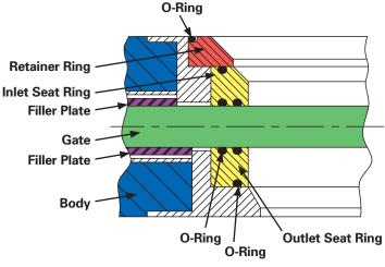
Tight machined tolerances of gate, filler plates and body limits spaces that could fill with plastic.
