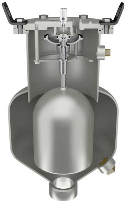
APCO ASU Combination Air Valves are made of 316 stainless steel and are available in 1-6" sizes with an operating range of 2 to 150 psi, or an extended range of 2 to 300 psi. They are available with flanged or threaded ends and meet the requirements of AWWA C512.
