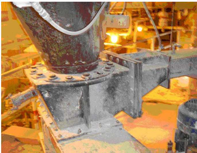
A specialized tapered body knife gate valve with a fabricated displacement pocket in the body which enables the valve to close against a standing column of dry, packed material.
