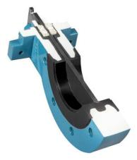
All wetted surfaces of DeZURIK KUL Urethane Knife Gate Valve Bodies are lined with urethane. The bonding process enhances the mechanical and abrasion resistance properties of the urethane, which creates a robust seat seal in harsh slurry services.
