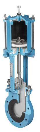
DeZURIK KUL Urethane Knife Gate Valves have a continuous bonded urethane liner throughout the entire body, chest, packing chamber and flange face area.
