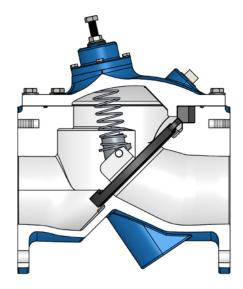
Also, subsequent wave patterns were more subdued and rounded. On-site closure noise (valve slam) and pipe displacement disappeared with the 100SR Spring Return.
