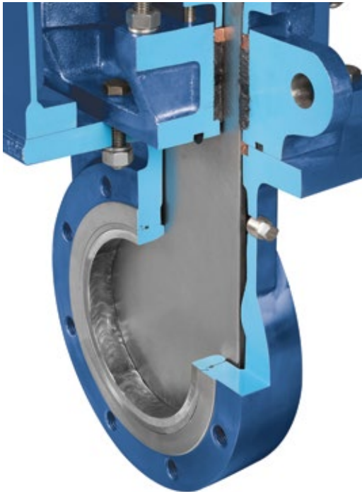
Purge ports in the chest area, cast lifting lugs and a robust packing system make this valve ideal for isolation service in high-pressure, high density slurry lines.
