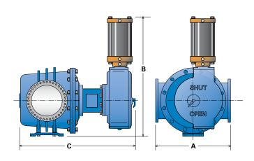
Torque unit (valve operating mechanism) complete with appropriate operator is shown in its customary vertical orientation, (perpendicular to pipeline), however, torque unit complete with operator may be rotated in any of 90° increments (parallel with pipeline) if so desired to suit installation requirements.
