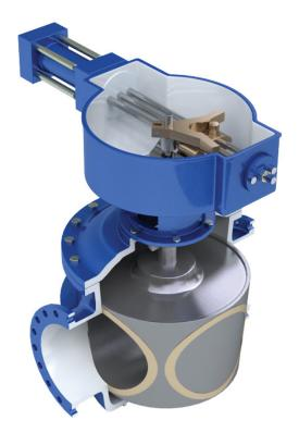
In operation, the plug is first lifted to separate the seat from the valve body seat. It is then rotated 90° to the desired open or closed position before being lowered to reseat in place. The body and plug seat are designed to form a secure, consistent and dependable closure.
