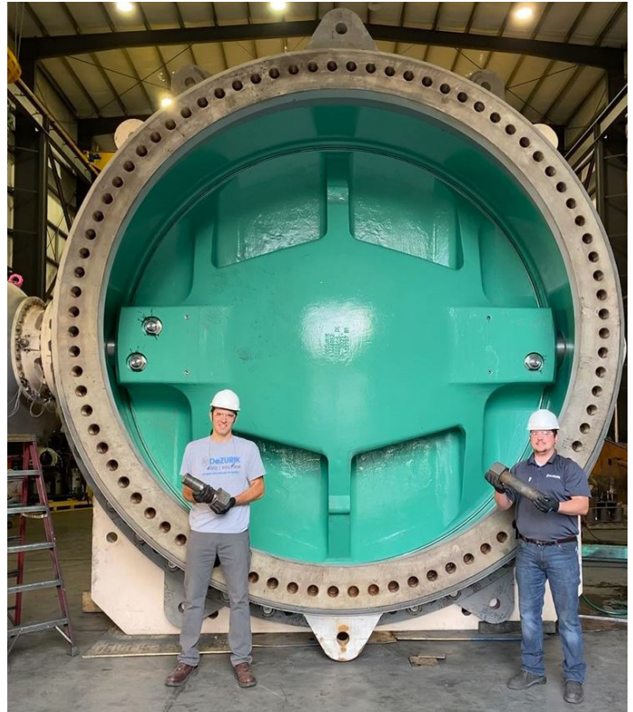
A 168" AWWA butterfly valve, the largest ever manufactured in North America, has fully flanged double flanges for exceptional strength.
